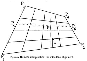
Given the control point coordinates the coordinates of P in the relative coordinate system which is defined as the fractional distance along opposite sides of the quadrilateral are desired. The relative coordinate w is the one required for alignment; the profiles are defined along the center-line of each lane and for inter-lane alignment the profiles need to be translated within the control quadrilateral to a common line. In order to determine w we introduce points  $P_5$  and  $P_6$  then,
