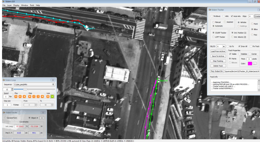
Fig. 3. The KOLAM user interface, showing the various subsystem widgets during a sample session for tracking moving and stationary objects, the lat-long position readout panel in the lower left, filename, ROI and zoom information in the status bar, interactive animation panel, assisted multi-object tracking panel on the right that also controls the display parameters for multiple trajectories and the original and stabilized trajectories trailing behind the two tracked objects.
