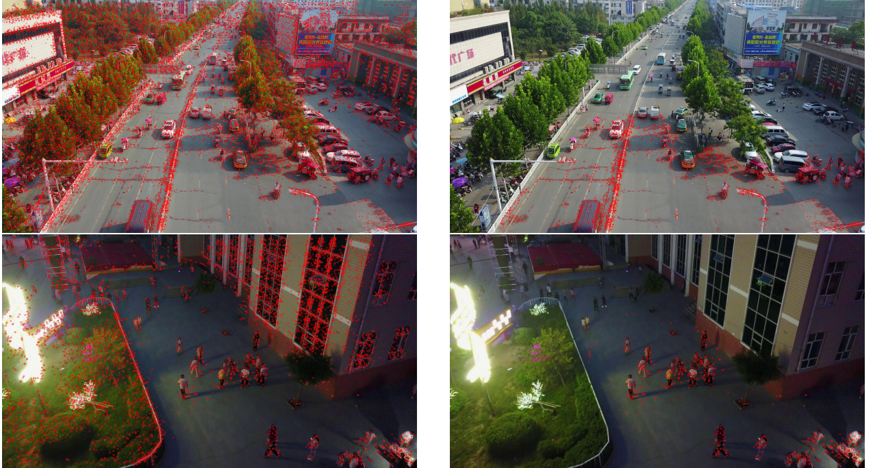
Figure 6. Keypoints extracted by SURF from a UAV captured frame from the video sequence uav0000148_00840_s and uav0000070_02088_s 24 respectively. Left: without plane segmentation. Right: using ground plane segmentation.
