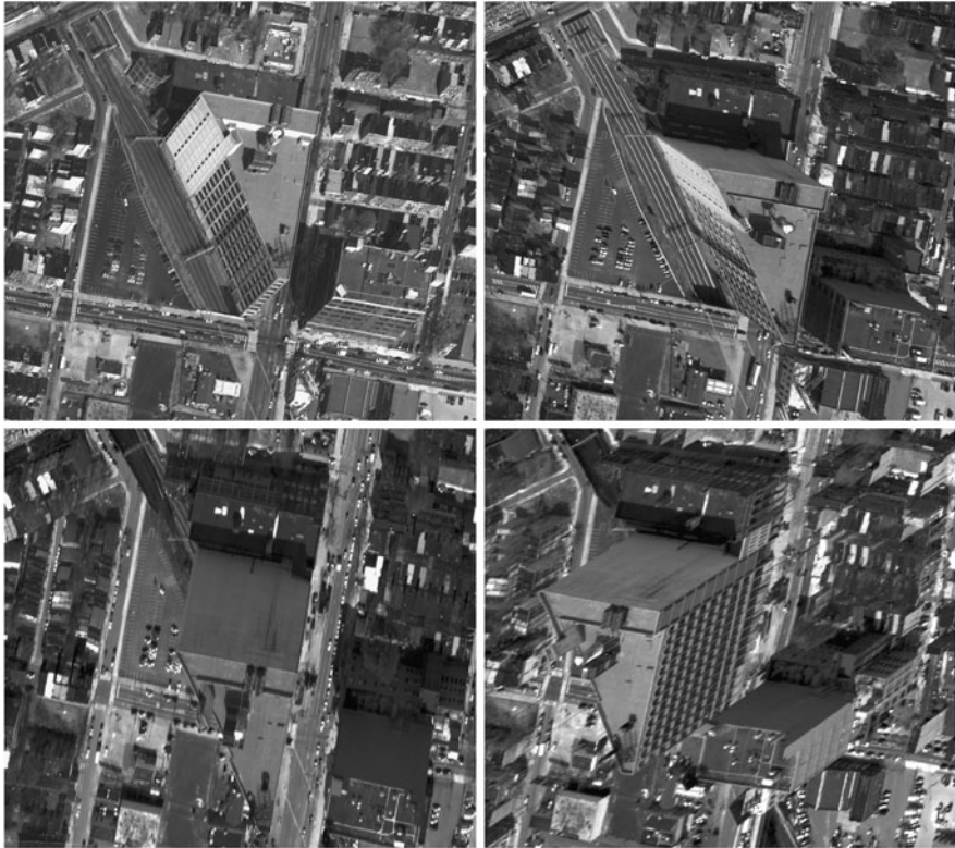
Fig. 4 The tall triangular building creates geometric occlusions of the road, ground-plane level structures, vehicles and pedestrians due to viewpoint induced wobble that is proportional to building height
