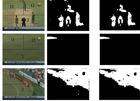
Figure 7. Row-1 shows pitch view: (a) Image (b) motion-mask (c) connected component image, Row-2 shows long view: (d) Image (e) motion-mask (f) connected component image, Row-3 shows boundary view: (g) Image (h) motion-mask (i) connected component image
